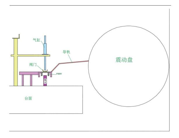
Sealing and vacuum: open the switch, sealing machine lifting and gas cylinder falling, sealing jaws pressed valve cover, vacuum machine starts vacuum, after vacuuming the lifting cylinder presses, making the valve and bottle fits, then the sealing cylinder presses so as to achieve sealing.
