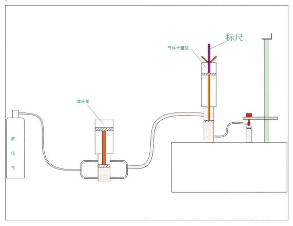
液化气: Liquefied gas 增压泵: Booster pump 气体计量缸: Gas metering pump 标尺: Scale
