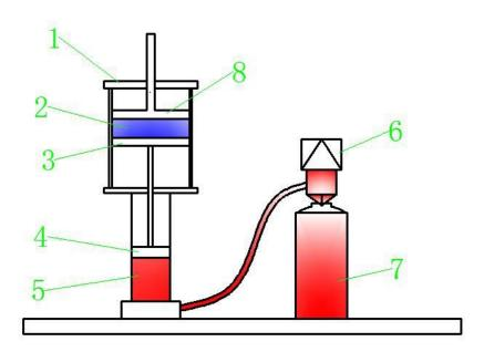
1. Filling metering cylinder; 2. Compressed air; 3. Power piston; 4. Filling piston; 5. Material; 6. Filler; 7. Aerosol can; 8. Metering control piston
