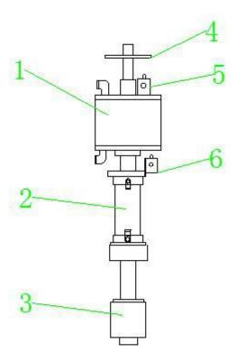
1.Closing cylinder; 2. Lifting cylinder; 3. Closing end; 4. Trigger of reset signal valve; 5. Reset signal valve; 6. Closing signal valve
