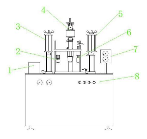
1. Transmission; 2. Liquid filler; 3. Liquid filling metering cylinder; 4. Closing cylinder; 5. Gas filling metering cylinder; 6. Gas filler; 7. Pressure gage; 8. Switch control area
