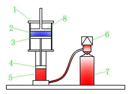
1. Filling metering cylinder; 2. Compressed air; 3. Power piston; 4. Filling piston; 5. Material; 6. Filler; 7. Aerosol can; 8. Metering control piston
