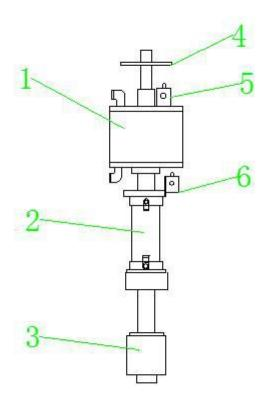
1.Closing cylinder; 2. Lifting cylinder; 3. Closing end; 4. Trigger of reset signal valve; 5. Reset signal valve; 6. Closing signal valve
